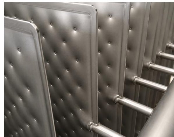
Gravity film distribution across the pillow plate surface
