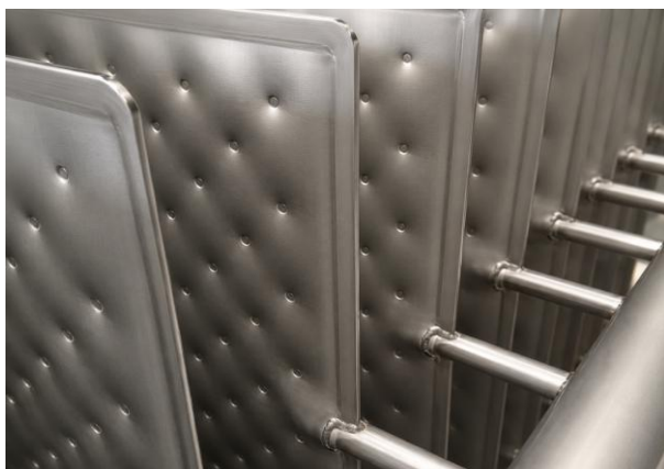
Pillow plate surface — gravity film distribution detail
